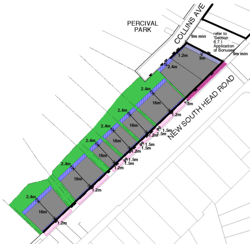
Ground floor level controls
