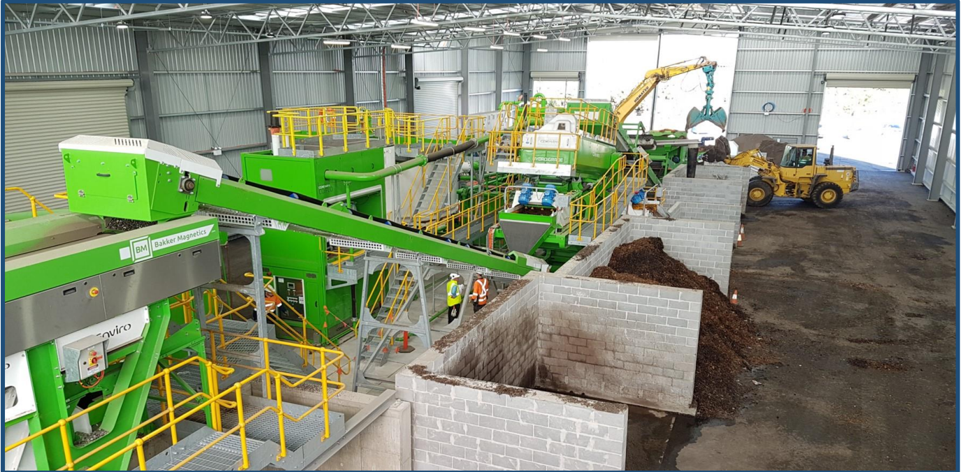
Figure 2. Downer's Detritus plant takes street sweepings and landfill, and turns this into materials used for manufacturing quality asphalt and building materials
