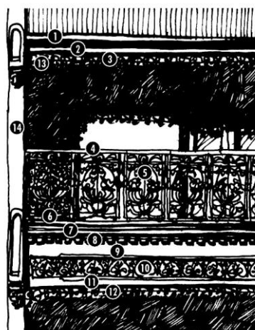
Figure 3.7 Typical Victorian terrace verandah elements.
