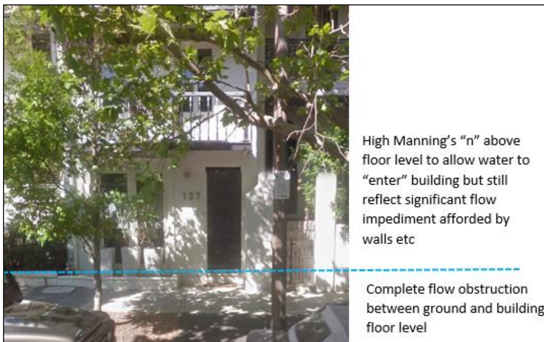
Plate 13 Conceptual representation of buildings in TUFLOW model
