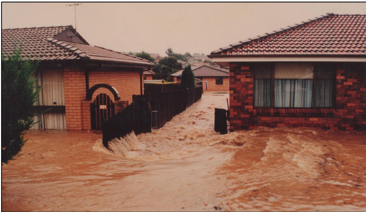
Plate 14 Example of paling fence causing a notable impediment and redistributable of overland flows
