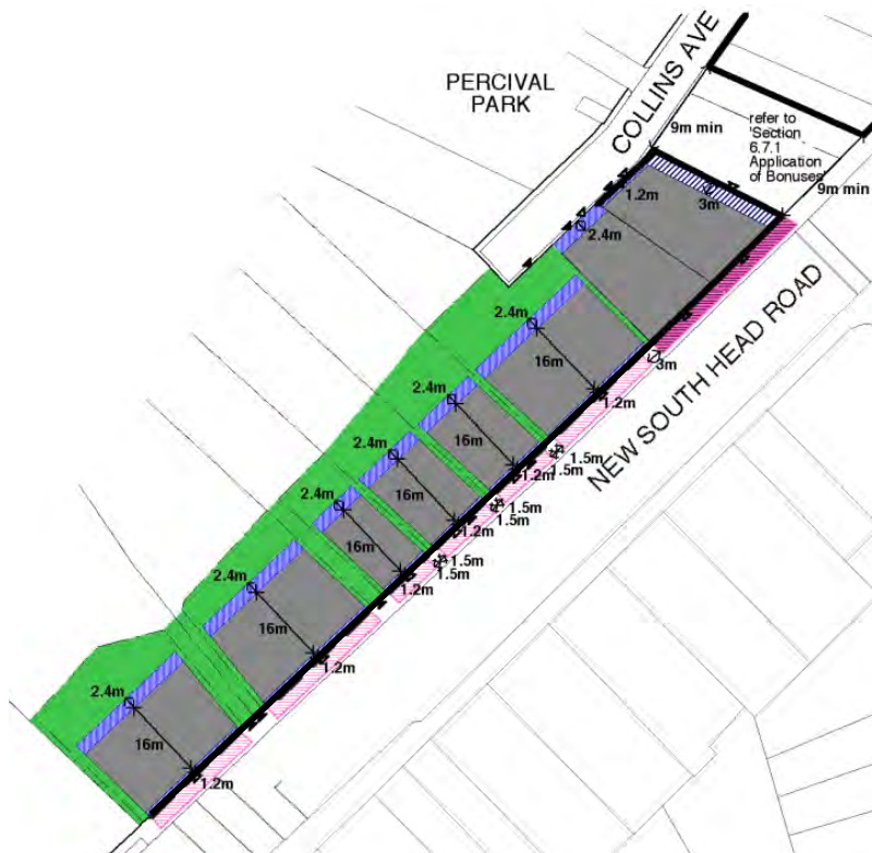
Ground floor level controls
