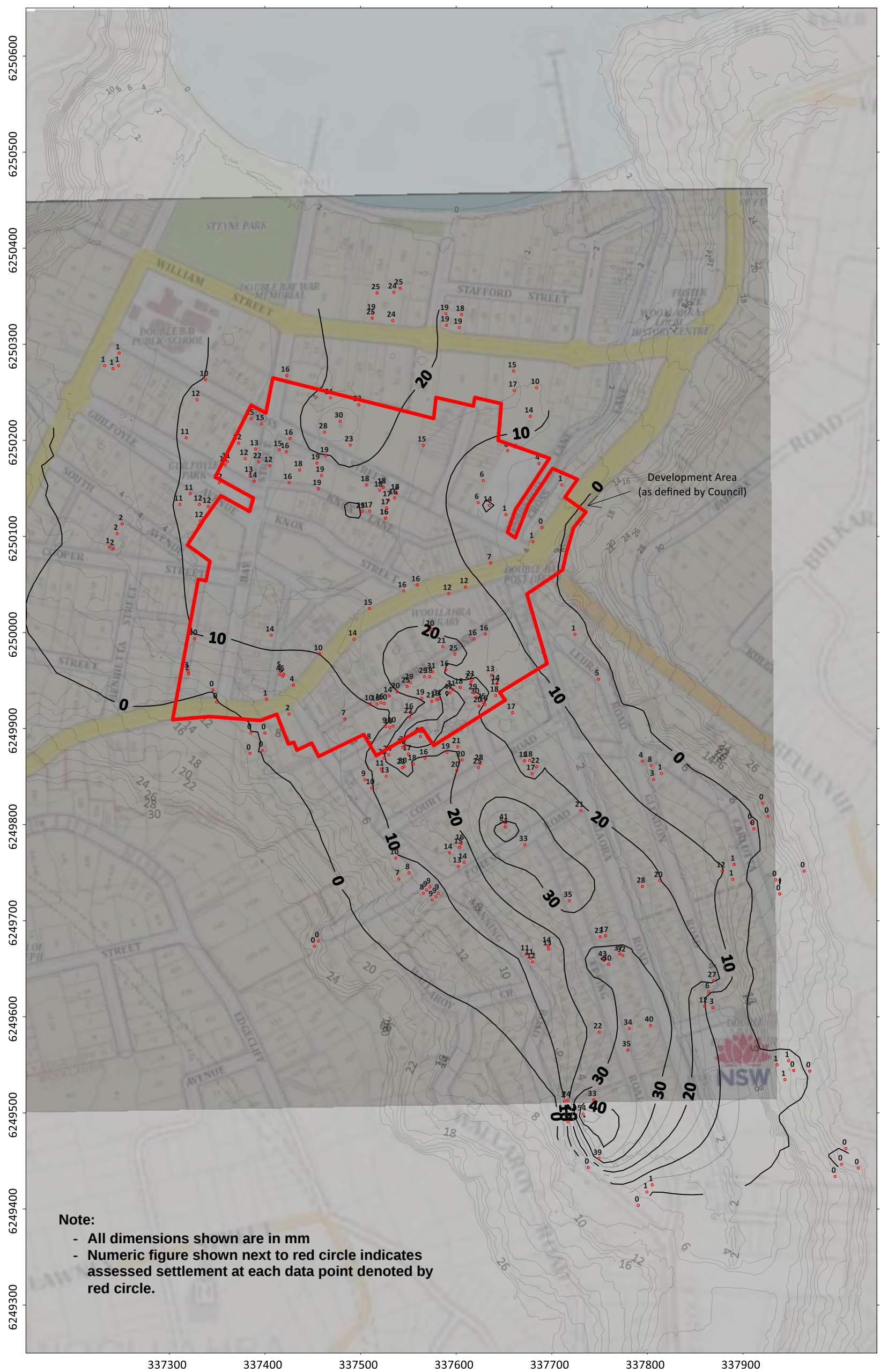
Figure 26 Contours of assessed settlement index for 1-m drawdown depth
