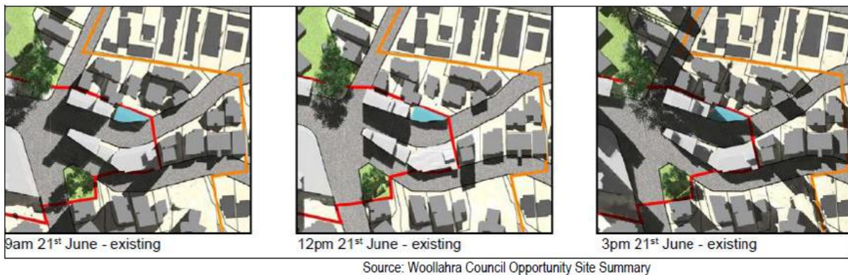
Figure 6: Shadow diagrams – Existing buildings
