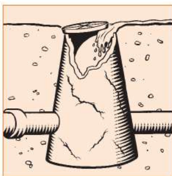
Hidden or damaged maintenance holes
