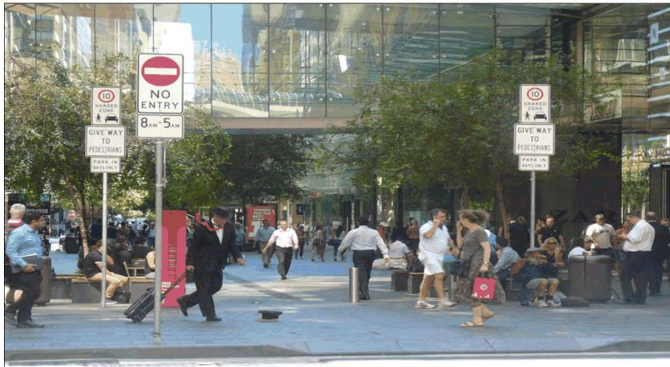
Figure 1. Photo and diagram of a Category 1 shared zone showing regulatory signage, typical layout and treatments. [Note: The No Entry sign is site specific] The photo may have been modified to demonstrate essential elements.
