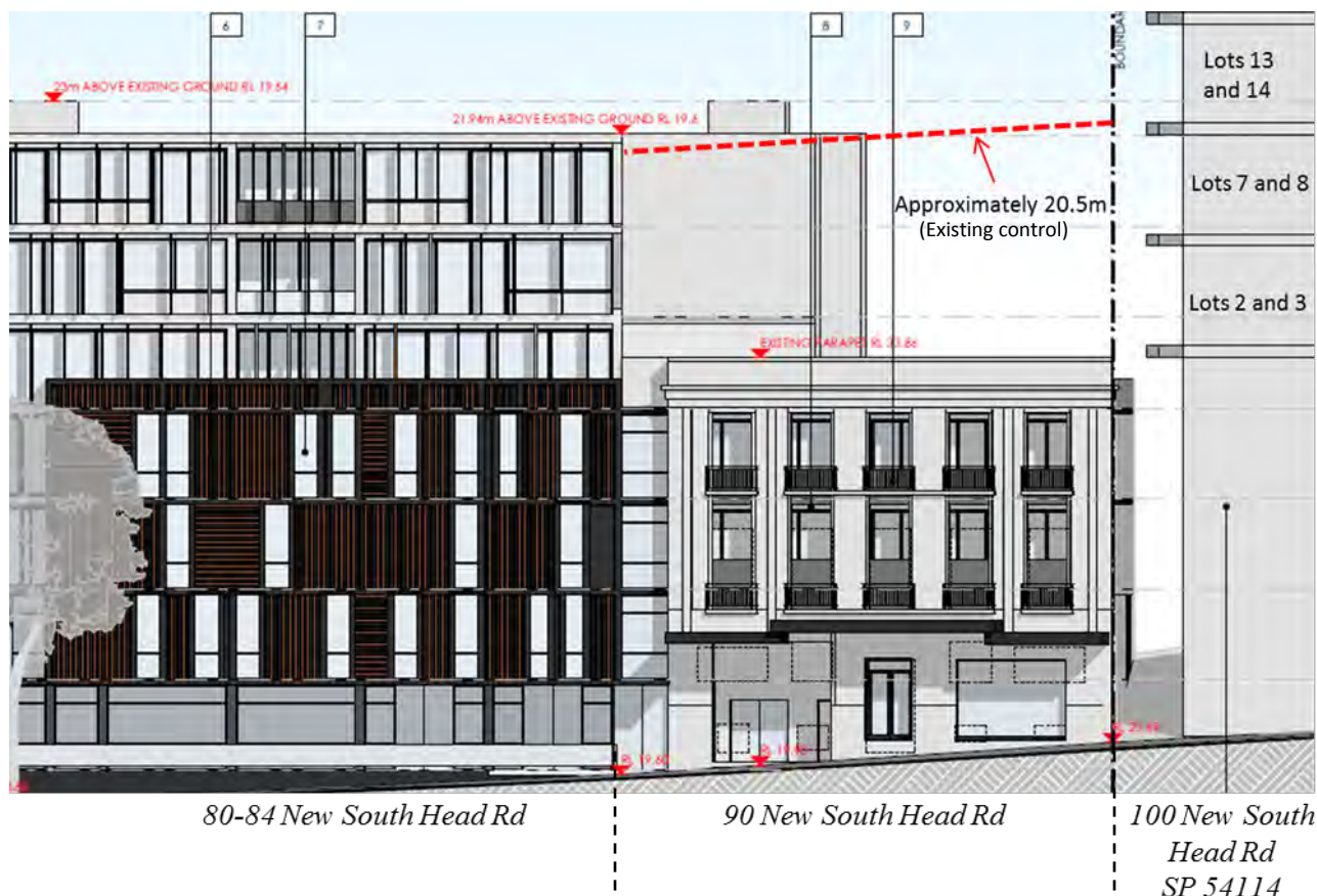
Figure 11: Comparison of concept plans, existing height limit and location of lots in SP 54114
