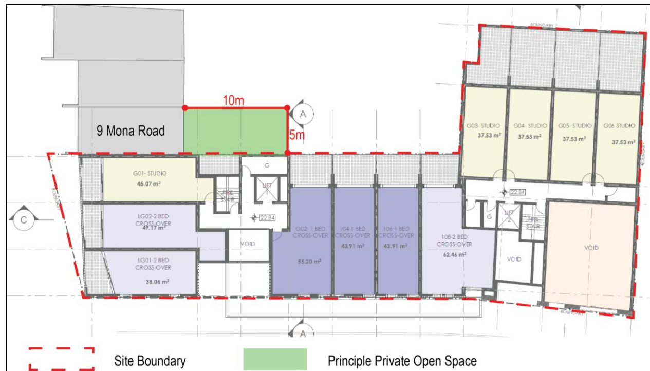
Figure 25: Proposed Building Separation – Ground Floor
