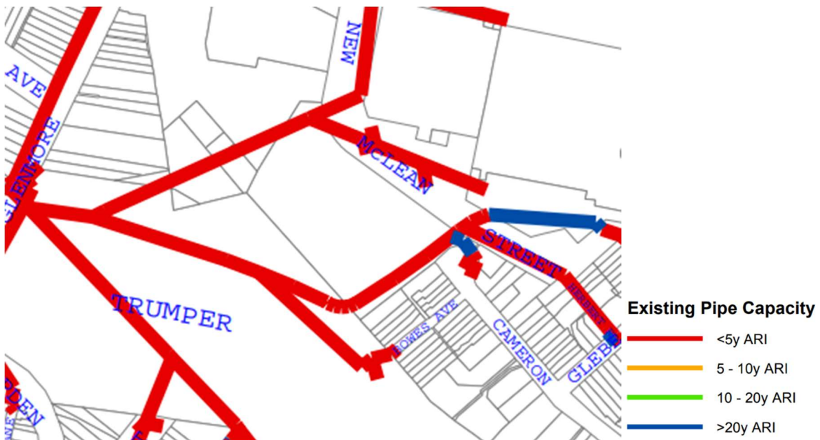
Existing Stormwater Infrastructure Capacity (Source: Rushcutters Bay Flood Study)
