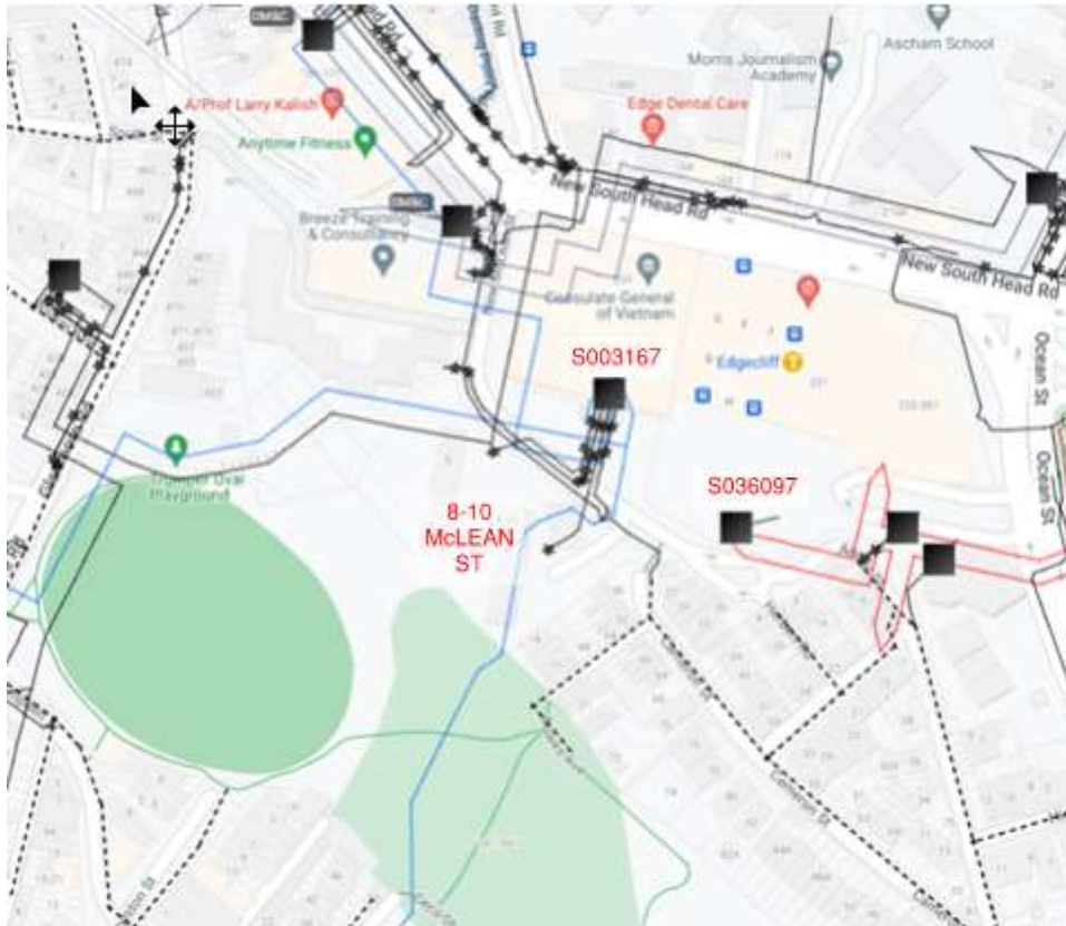
Ausgrid WebGIS extract showing LV network
