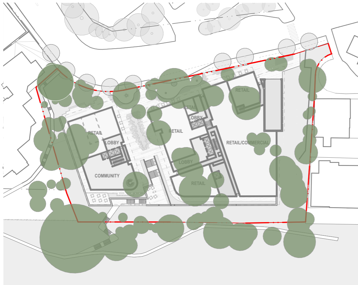
Existing Tree Canopy Coverage 37%
