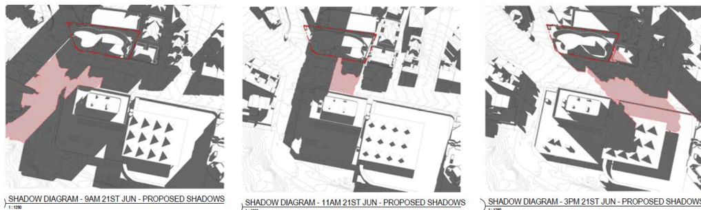
Figure 8: Sample of existing shadows (grey) and from a new building on the site (pink) (Source: Planning Proposal Concept Report, GroupGSA 2021)
