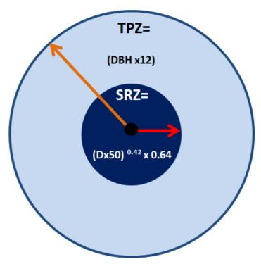
FIGURE 10: A REPRESENTATION OF THE CALCULATIONS REGARDING TREE PROTECTION ZONES (TPZ) AND STRUCTURAL ROOT ZONES (SRZ).
