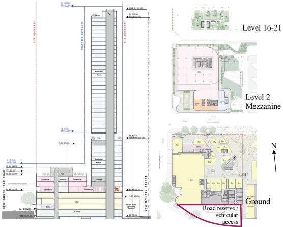
Figure 2: North-south section looking east (L), various plans (R)
