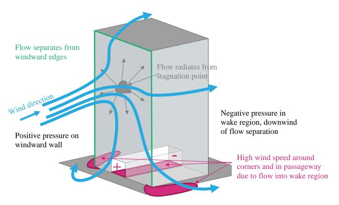
Figure 5 Schematic wind flow around tall isolated building
