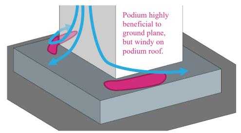
Figure 6 Schematic flow pattern around building with podium
