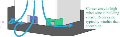
Figure 9 Schematic of flow patterns around isolated building with ground articulation
