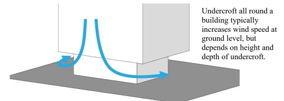
Figure 8 Schematic of flow patterns around isolated building with undercroft
