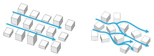
Figure 11 Schematic of flow patterns through a grid and random street layout
