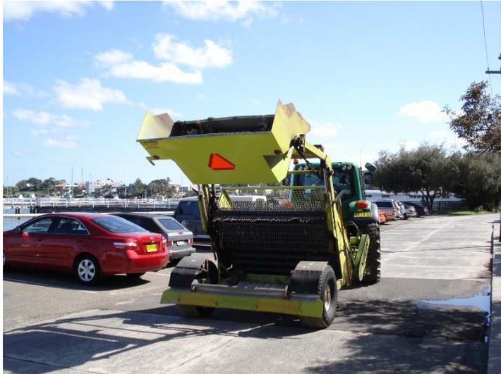
Mechanical rake collects waste which can be deposited directly into a garbage truck, or utility.
