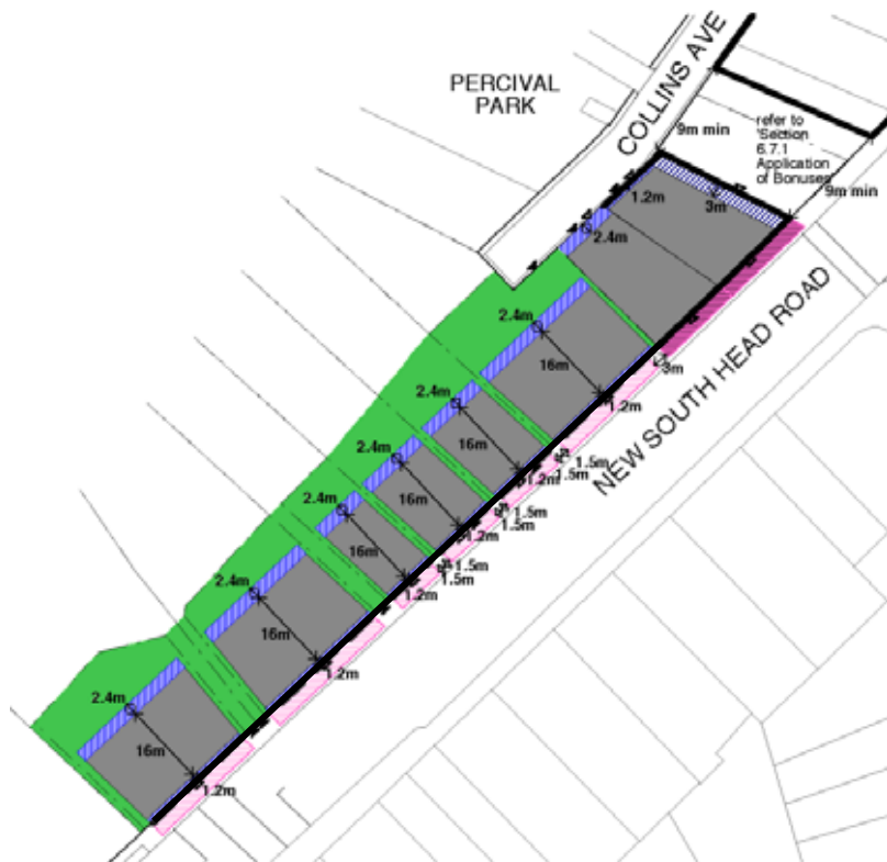
Ground floor level controls
