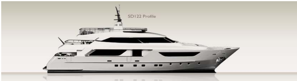
FIGURE 2. This typical 37 m long motor vessel is approximately 8m high above the water line excluding the funnel and mast.
