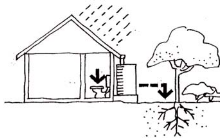
Fig 5.17 rainwater tanks to supply water for cooling systems, toilets, outdoor cleaning or gardens
