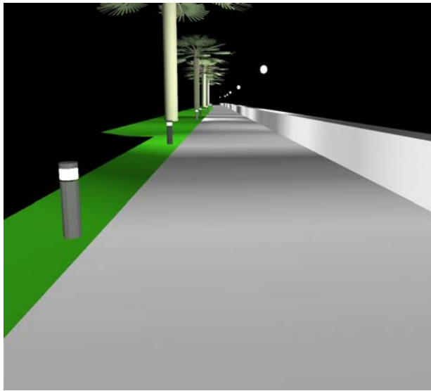
Light simulation with bollards at 10m spacing
